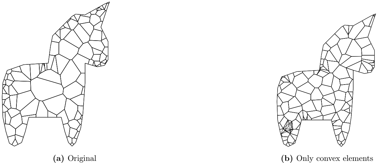
Figure 7.9: Partitioning nonconvex elements in the unicorn mesh
