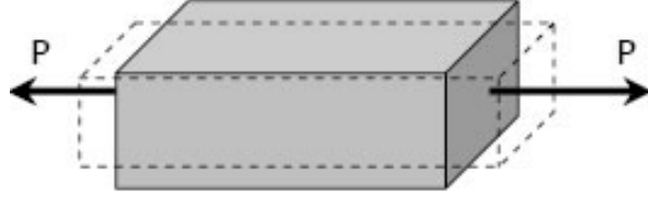
Figure 2.10: Representation of the Poisson effect
