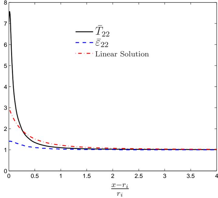
Figure 7: Variation of the normalized stress and strain near the hole.
