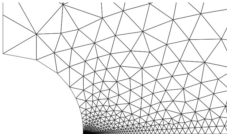
Figure 3: Mesh near the surface of the hole.
