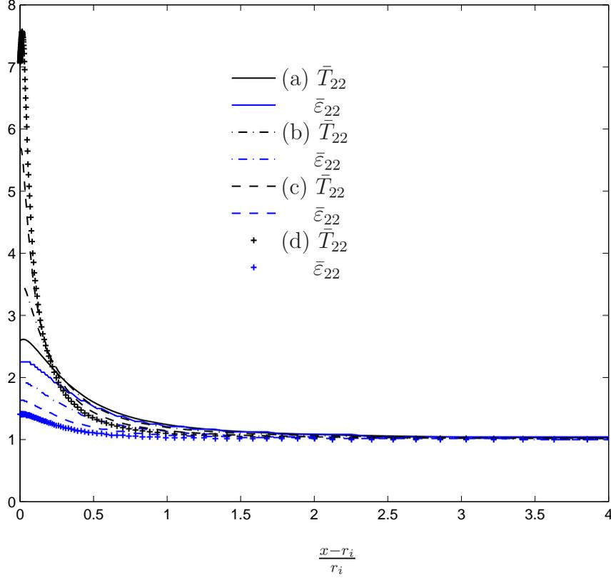
Figure 8: Behaviour of the normalized stress and strain near the hole for different values of the external load  $\sigma_\infty$  Pa (a) 0.25, (b) 0.5, (c) 0.75 and (d) 1.
