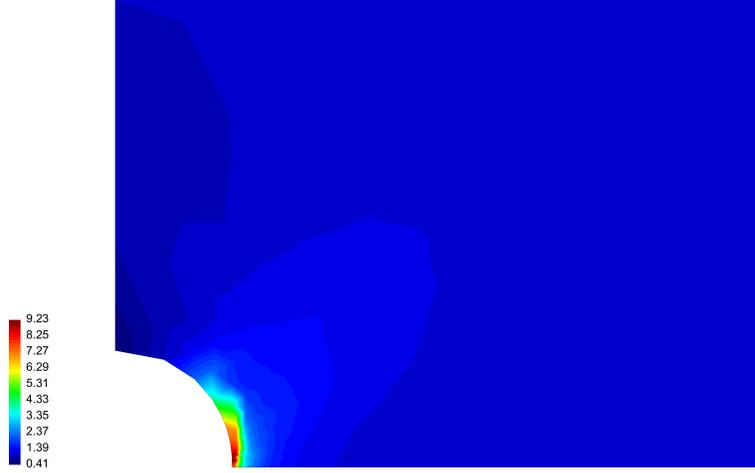
Figure 6: Contour plot for the stress  $T_{22}$ . Stress in [Pa].
