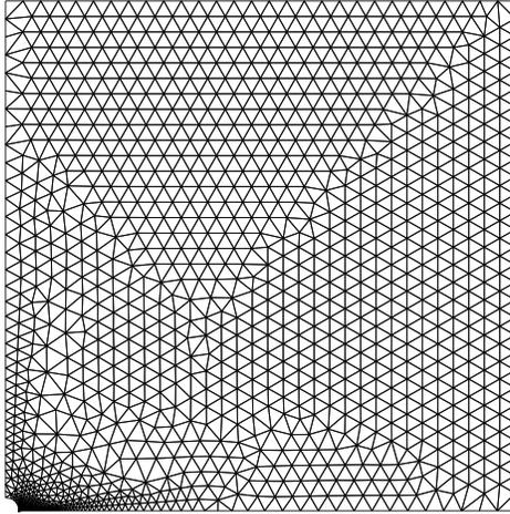
Figure 2: Mesh for a quarter of the whole plate.
