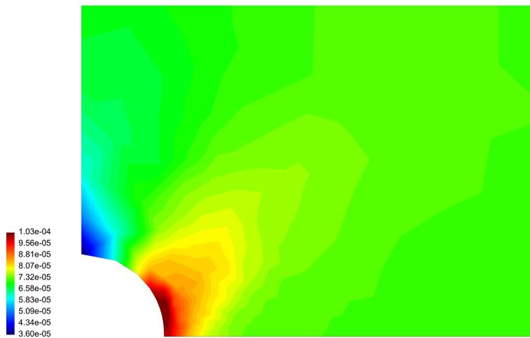
Figure 5: Contour plot for the strain  $\varepsilon_{22}$ .
