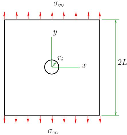
Figure 1: Plate with an hole under uniaxial boundary traction.
